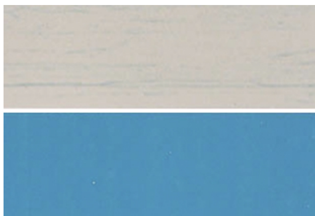
Figure 4. Optical photomicrograph of an air-dried oriented film prepared from a solution of 1 (11 wt%) in aqueous 16.5 N HCOOH: (top) polarization axis of incident light parallel to the shearing direction, and (bottom) polarization axis of incident light perpendicular to the shearing direction (200×, single polarizer).
